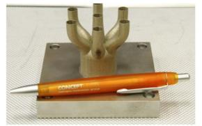
Fig. 53 - Polycarbonate wiring conduits made by fused deposition modeling. Courtesy Stratasys and Bell helicopter [48]
