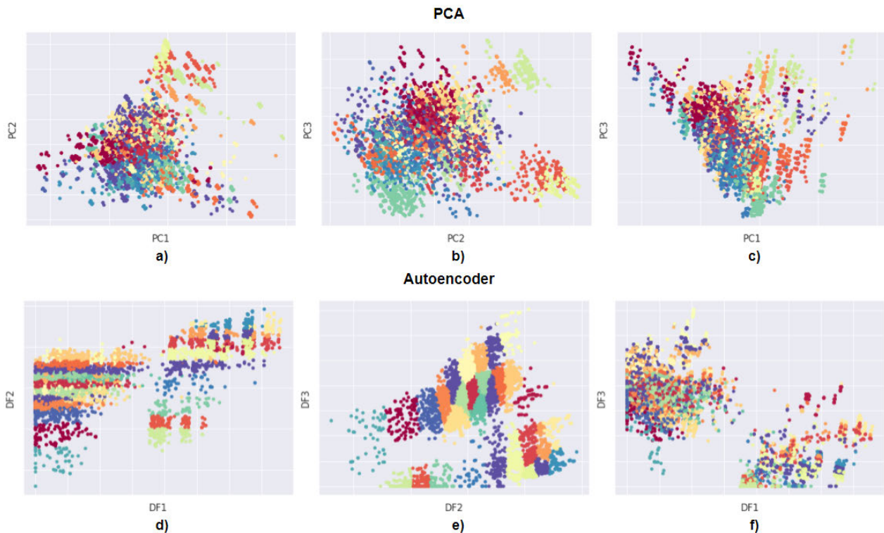
FIGURE 2. Clusters projected onto a reduced feature space containing binary combinations of the extracted features. PCA (top), Autoencoder (bottom).
