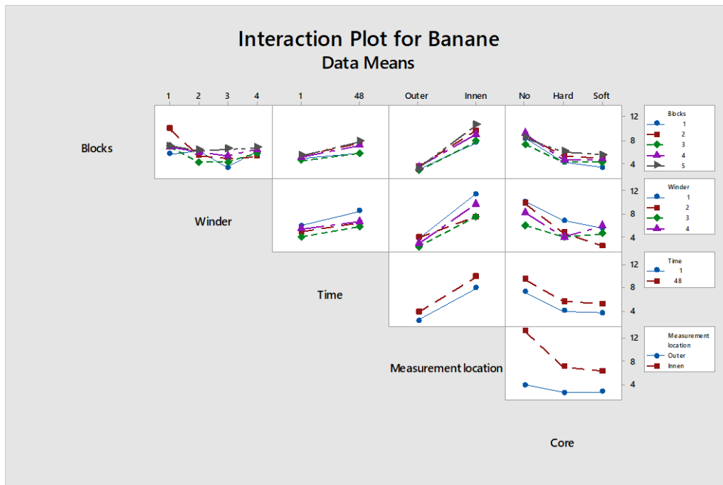
Figure 5-14: Winding test no.2 interaction plot
