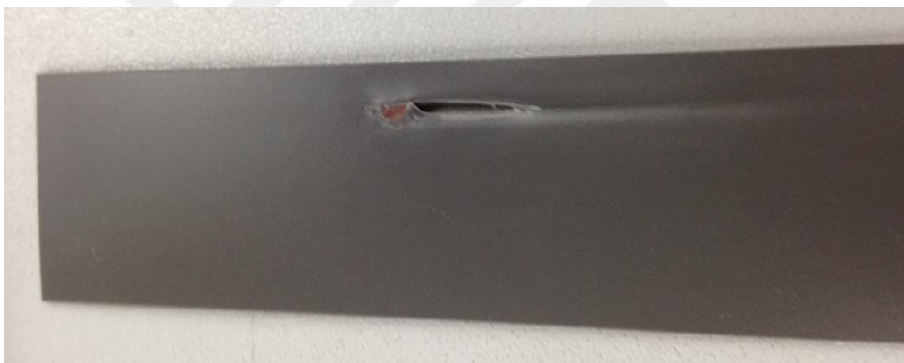
Figure 6-2: Teared edge band due to macro foreign substance
