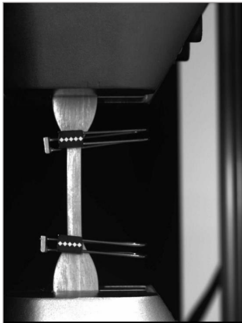
Figure 29 ASTM 638 resin specimen tensile testing
