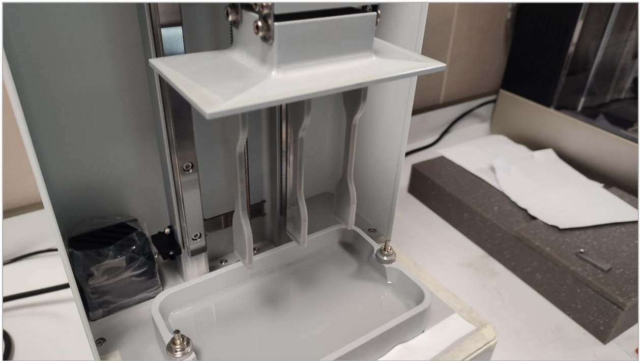
Figure 27 Printed ASTM 638 tensile specimen
