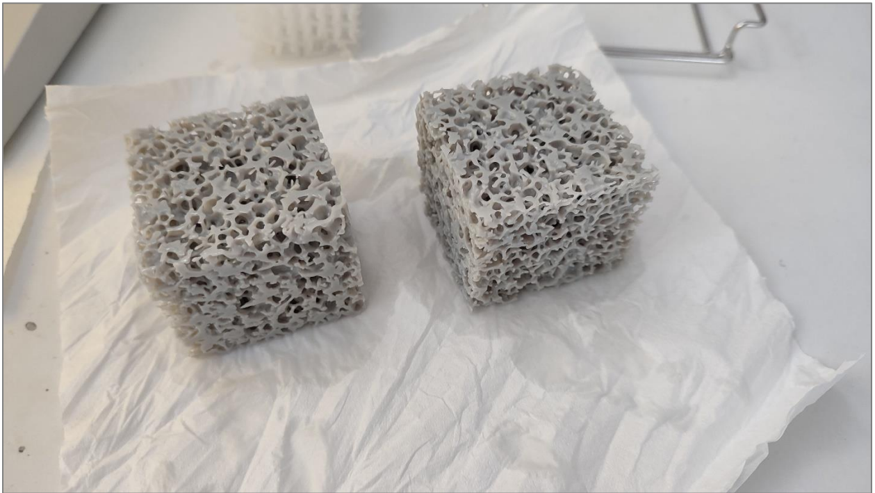
Figure 20 two merged (10ppi+3ppi) samples
