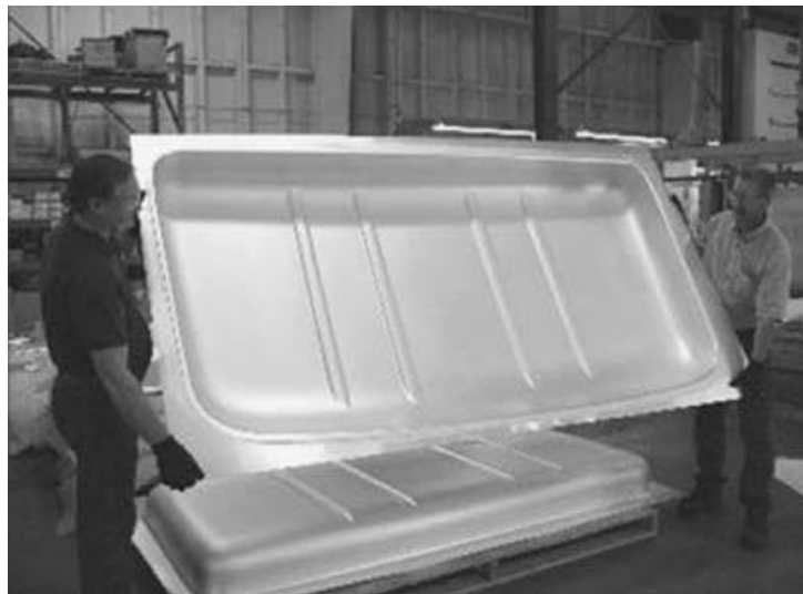
Figure 2.6: Simple female forming example for large one-piece truck cab roof in SP5083 alloy (Barnes, 2007)
