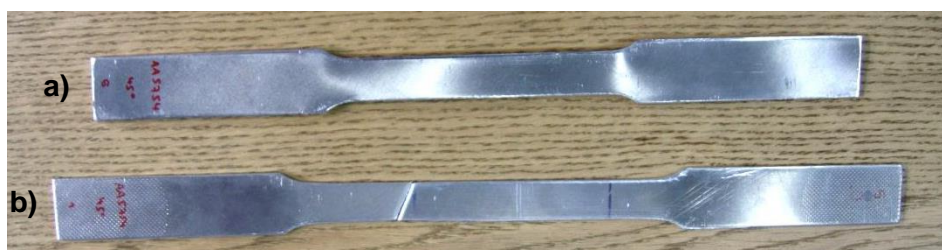
Figure 4.4: AA5754-H22 45° tensile test specimen: a) before the tensile test b) after the tensile test
