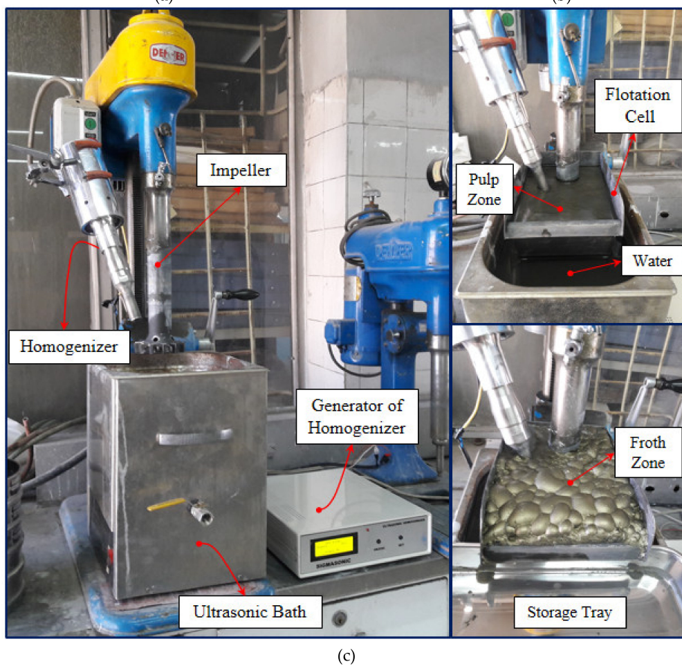
Figure 2. Schematic representation of the (a) 2D experimental setup for the flotation tests, (b) 3D overview of the flotation cell, and (c) laboratory design of the integrated cell with the ultrasonic bath and the homogenizer.
