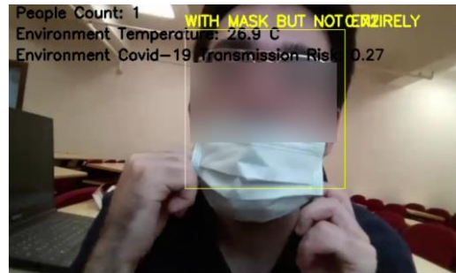
Fig. 8. Experiment 2 UAV image file with mask wearing rate from trained machine learning model and indoor temperature information from UAV sensor.
