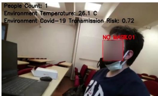
Fig. 6. Experiment 1 UAV image file with mask wearing rate from trained machine learning model and indoor temperature information from UAV sensor.
